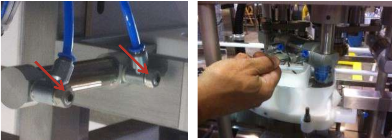
Figure 28 Adjusting air flow control screws on seam station air cylinder
