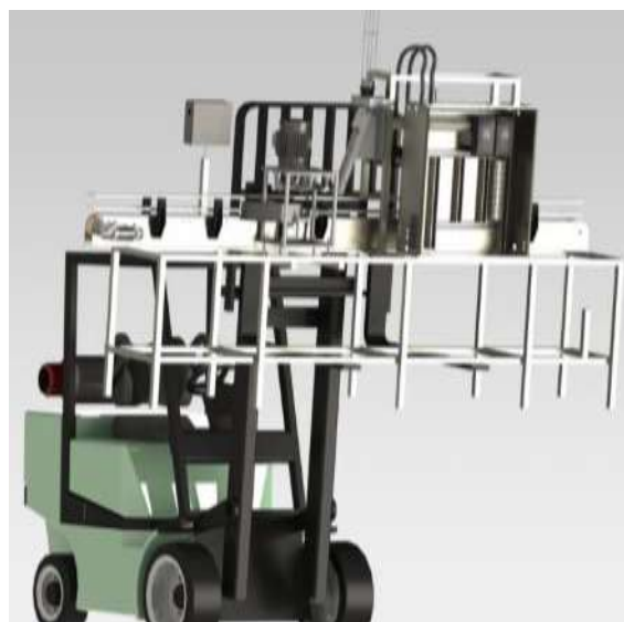
Figure 5 Forklift moving Cask ACS into position
