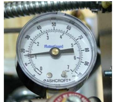
Please record the system pressure at the start-up of your Haskris system. Whenever the pressure increases 5-6 psi (0.3 - 0.4 Bar) above the initial start-up pressure, you should clean the strainer.
