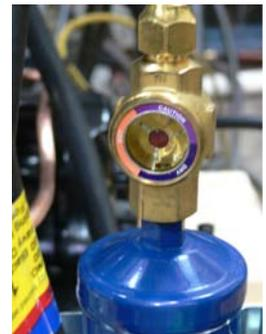
**Note:** It is normal to see bubbles immediately after the compressor turns on, and immediately after it turns off. The sight glass should be clear when the system is continuously running.
