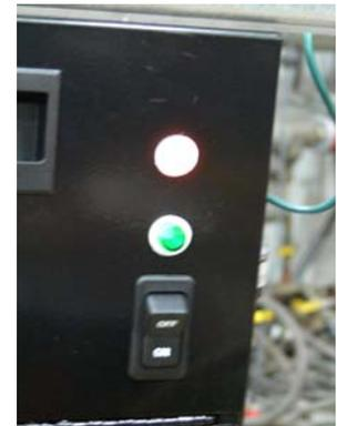
Systems with 5, 6 or 9 gallon (19, 23 or 34 liter, respectively) tanks also have a liquid-level interlock relay. If the water level drops, the liquid level switch opens and the relay will shut the system down (refer to the wiring diagram located inside your Haskris system, on the tank).
