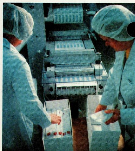
Cartoning of medical disposables after discharge from the R-7000.
