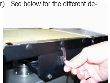
Version "A" quick-release latch
