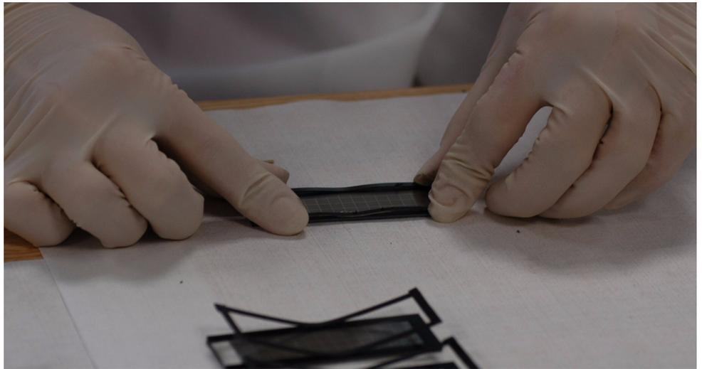
The OpenArray plate is now sealed, framed, and ready to insert in the OpenArray NT Cyclor.
